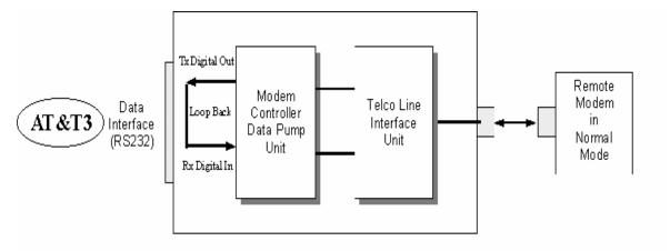
Figure 3 PERFORM LOCAL DIGITAL LOOPBACK
